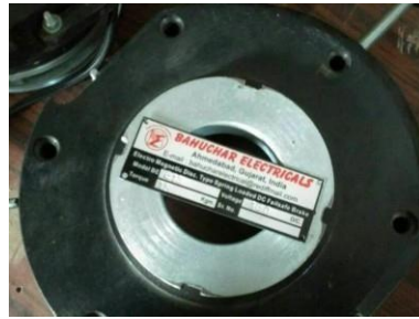
Electrical Brake Ac & Dc
