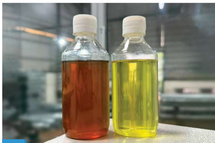
04 Before & After Polishing of Plastic Pyrolysis Oil
