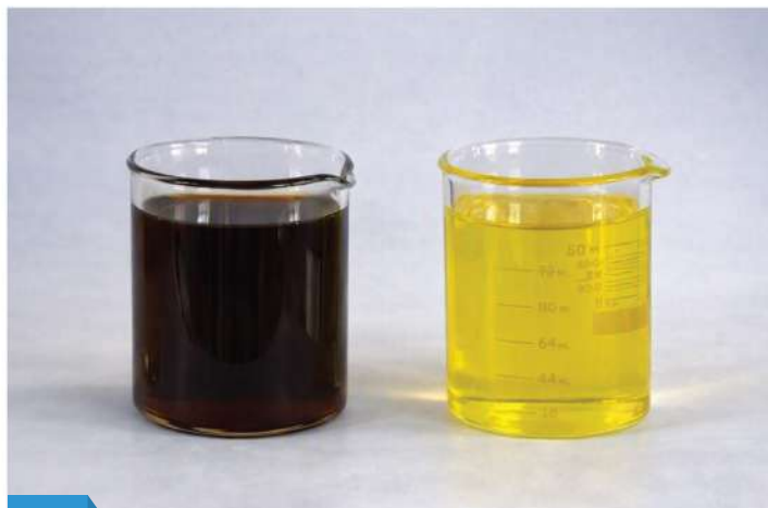
01 Before & After Polishing of Lube Oil
