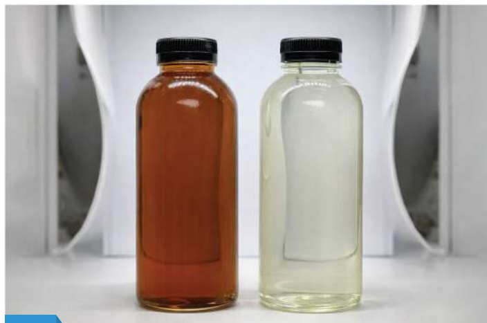
02 Before & After Polishing of Transformer Oil
