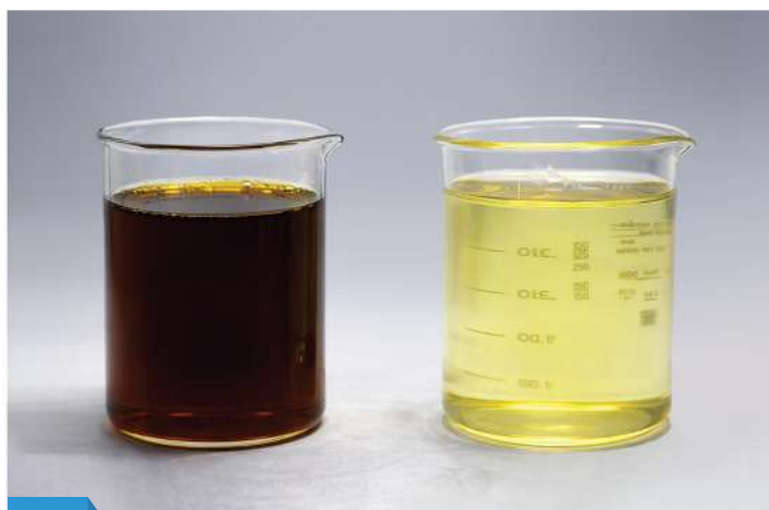
03 Before & After Polishing of Light Diesel Oil
